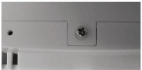
After undoing the screw pull it forward until the screw stops moving, then carefully separate the two halves of the case by gently pulling in an upwards direction. Once the case has been separated, the batteries should be visible:
