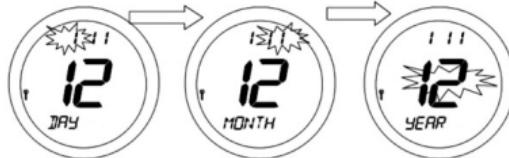
Confirm the setting using the OK key, or Press the Arrow key to return to the previous screen display. The next menu screen allows you to set a temperature setting. This temperature is the maximum temperature that the heating system will operate at once the previously set service date is reached.
