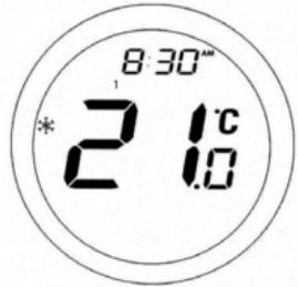
If the ST620RF is operating in FROST mode the LCD will not indicate MANUAL or AUTO, but will display both the room temperature and also the FROST mode indicator.
