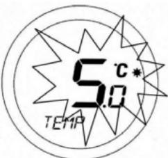
Pressing the Touch Ring will change the display to show the current temperature setting, but this setting cannot be adjusted while in this mode.
