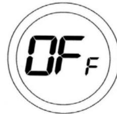
As all functions except sampling the battery voltage are disabled in OFF mode, it is recommended that you replace the ST620RF batteries as soon as possible to restore normal operation.
