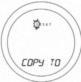
After entering the settings in Programmes 1 to 6 for Monday, the ST620RF display will change to display a COPY TO screen. On this screen, scroll to the day that you want to copy the settings to using the Touch Ring, and then confirm this by pressing the OK key. The ST620RF will then move to the next day and ask if you would like to copy again.
