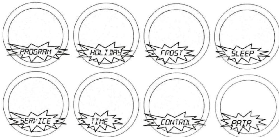
You can scroll through the menus in either direction (forwards or backwards) depending on the direction you move your finger around the Touch Ring. The menus are displayed in the order shown in the picture above.
