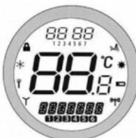
After two seconds, the ST620RF will then operate in NORMAL mode and display the current room temperature, with the RCC indicator flashing.
