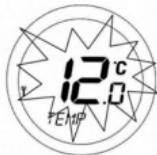
The temperature is set by scrolling the Touch Ring to the desired setting, then confirming with the OK key.
