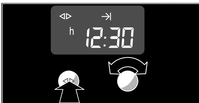
The appliance switches off automatically at the time set for the end of operation.
