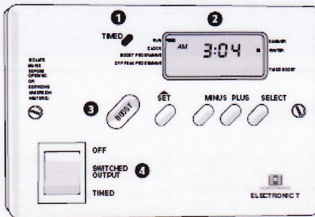
**LCD Display.** The LCD display allows the user to view the current time and set programme times.
